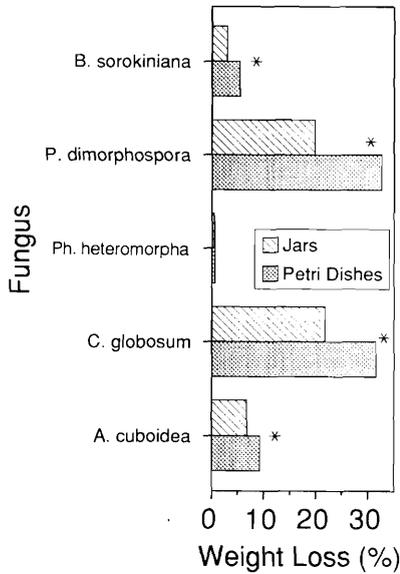
FIG. 2. Comparison of jars (containing 20 mL reduced nutrient agar) with Petri dishes (35 mL) as decay chambers, using thin mesh and birch blocks. Asterisks indicate significant differences according to a *t*-test ( $P = 0.05, n = 11$ ).
