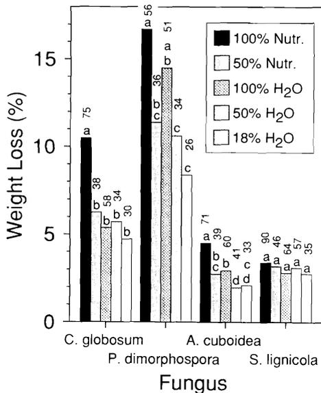
FIG. 3. Comparison of various methods of soaking birch blocks in a reduced nutrient agar system. Bars in a cluster with the same letter are not significantly different according to Scheffé's multiple-range test ( $P = 0.05, n = 11$ ). Numbers over the bars are the postdecay moisture contents. Incubation time was 6.5 weeks.
