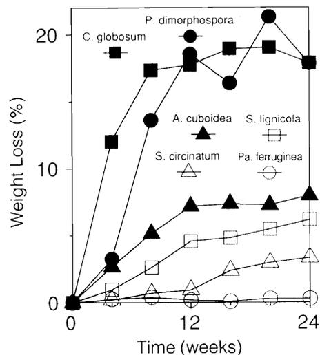
FIG. 1. Changes in weight loss of birch blocks during exposure to six soft-rot fungi. Blocks were incubated on a thin mesh over 20 mL reduced nutrient agar. Each point is the mean of 11 replicates.
